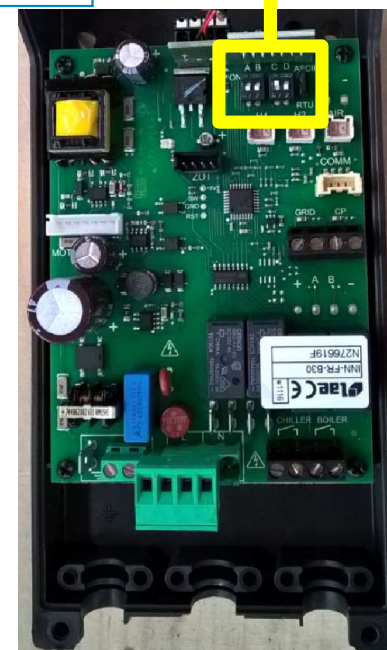
Control panel in performance mode with DIP switch A on (Default values)
